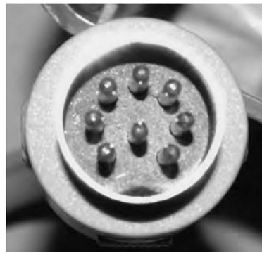
The steam generator connector
